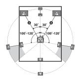
When placing two surround back speakers (The angle **B** should be the same)
